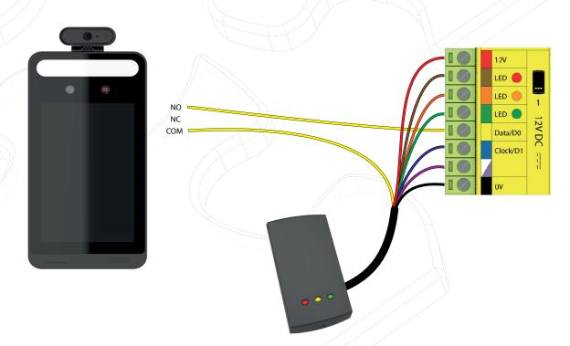
The default door lock delay on the Genie reader is 3 seconds. To allow sufficient time for the user to present their token to the Paxton reader, you may wish to increase this via the menu on the Genie reader.
