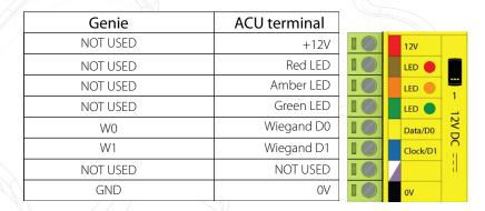
Ensure any unused wires are safely terminated.
