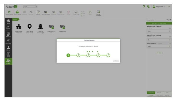
4. Once the local master comes online, all other Paxton10 hardware on the new site (the local subnet to which the local master is connected) will be detected by the master controller. These devices will appear in the device panel on the right-hand side, ready to be bound in the usual way.
