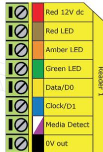
**Ensure any unused wires are safely terminated.**
